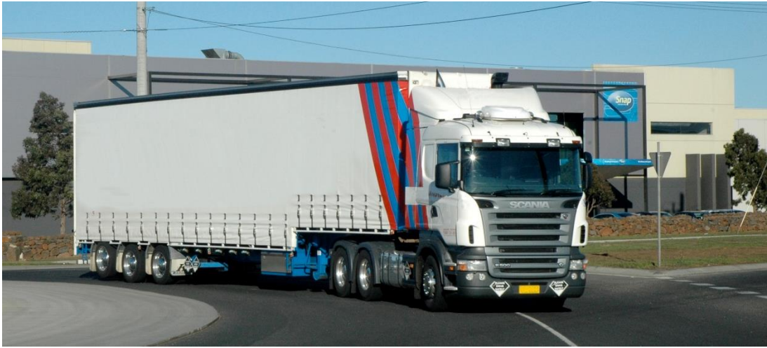
Figure 1: A photograph of a prime mover and semi-trailer combination, a common prescriptive heavy vehicle in Australia
